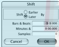
Figure 4-13: Use the Shift dialog box to adjust for the latency of the M-Box.
